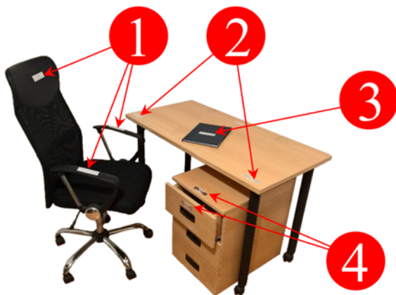
Fig. 6 Various objects of interest tagged: (1) Chair with 3 tags attached, (2) desk with 2 tags attached, (3) book with a single tag, (4) desk drawer tagged with 2 tags attached
